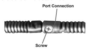
10. Check that the screw has secured the Drum Cable to the Replacement Cable. Look at the other side of the Port Connection. The bottom of the screw should be flush with the rim of the screw hole.
